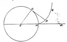
Let S be the centre of a circle, APQ a portion of the involute, OP = OA the portion of the string unwound. Let SO = a,  $OSA = \phi$ , and let x, y be the co-ordinates of P, the origin being at S, and SA the direction of the axis of x.
